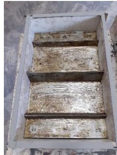
Figure 2: ASTM C1579 concrete slab mould used in the research
