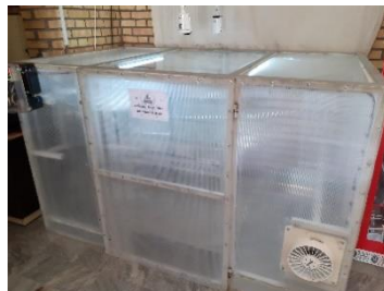
Figure 3: The atmospheric simulating chamber used in research
