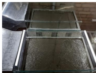
Figure 4: Concrete samples under testing in the atmospheric simulating chamber
